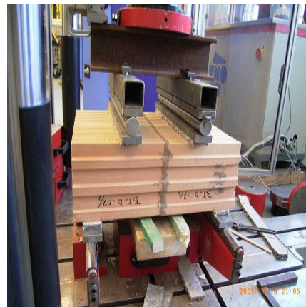
figure 1: finite-elements-model of a terraced house figure 2: four point bending test arrangement of TNO
