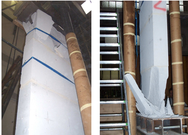
figure 8: Destroyed test specimen (KS-XL-PE)
