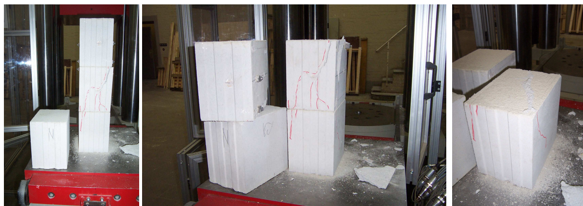
figure 7: Destructed joint of a test item (KS R)
