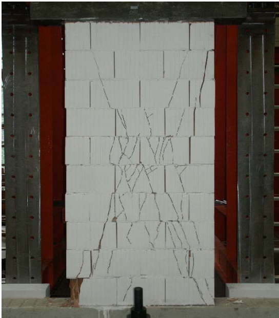
figure A8-1: crack pattern of test No. 8
