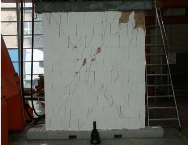
figure A4-2: crack pattern of test No. 4
