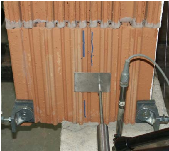
figure A25-1: first crack at the face side of test No. 25
