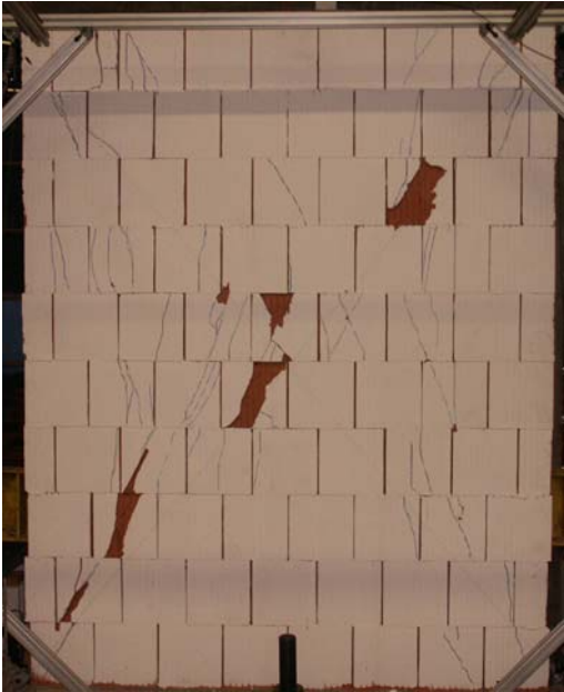
figure A24-2: crack pattern of test No. 24
