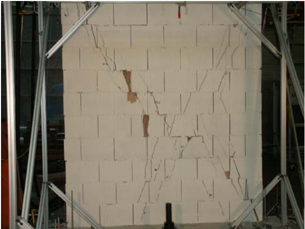
figure A6-2: crack pattern of test No. 6
