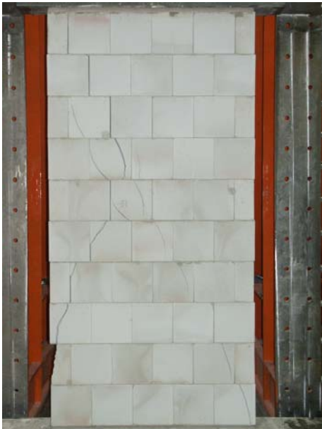
figure A17-2: crack pattern of test No. 17
