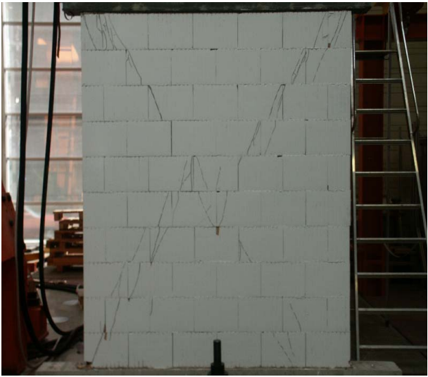
figure A10-2: crack pattern of test No. 10
