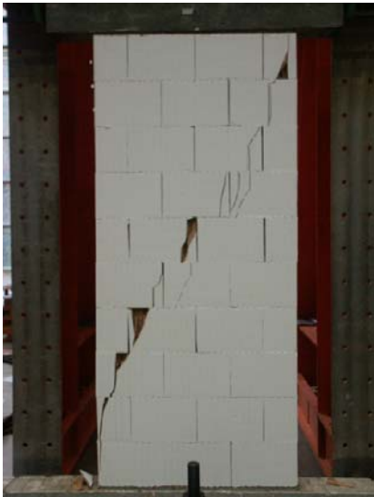
figure A13-2: crack pattern of test No. 13
