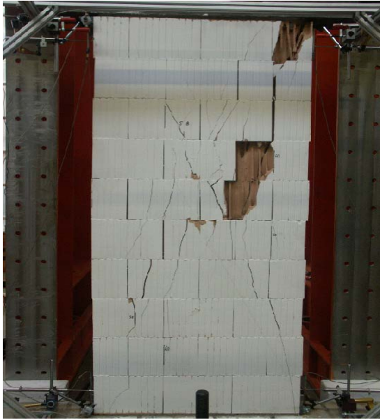
figure A7-2: crack pattern of test No. 7
