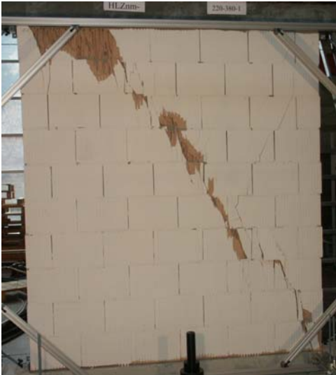
figure A1-2: crack pattern of test No. 1
