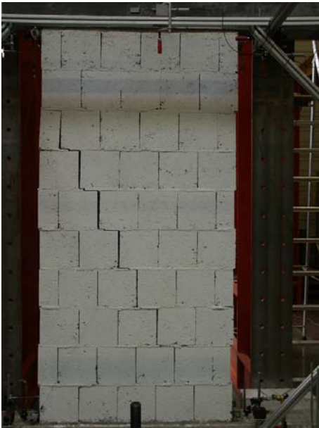
figure A20-1: crack pattern of test No. 20
