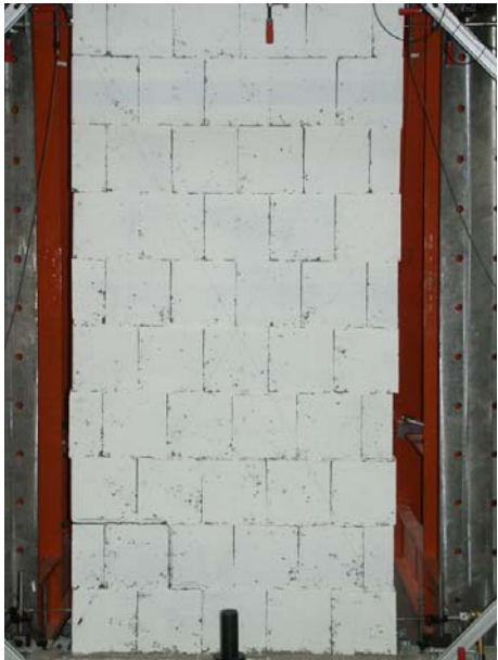
figure A22-2: crack pattern of test No. 22
