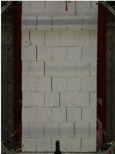
figure A18-1: crack pattern of test No. 18
