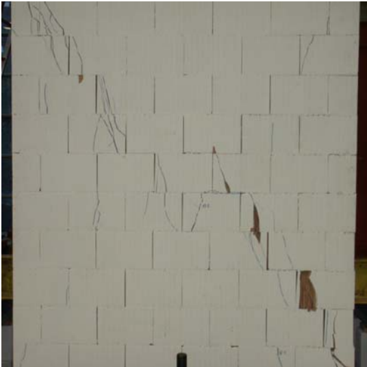
figure A1-2: crack pattern of wall No. 1
