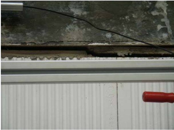
figure A6-2: opening of the had joint of wall No. 6
